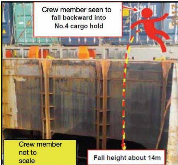
A container vessel was in the process of loading. At one point, a crew member was seen walking on the raised catwalk adjacent to number 4 cargo hold, which was open and empty. It was early morning and a fine dew had wetted most of the steel surfaces of the vessel.
